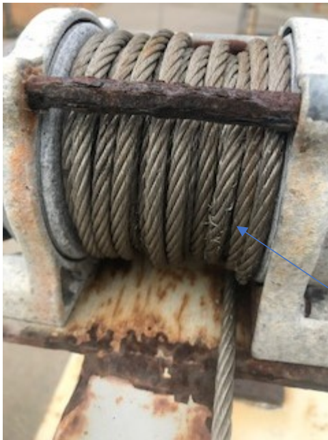
Figure 4 Cable replacement is needed and would exceed the value of the equipment.
