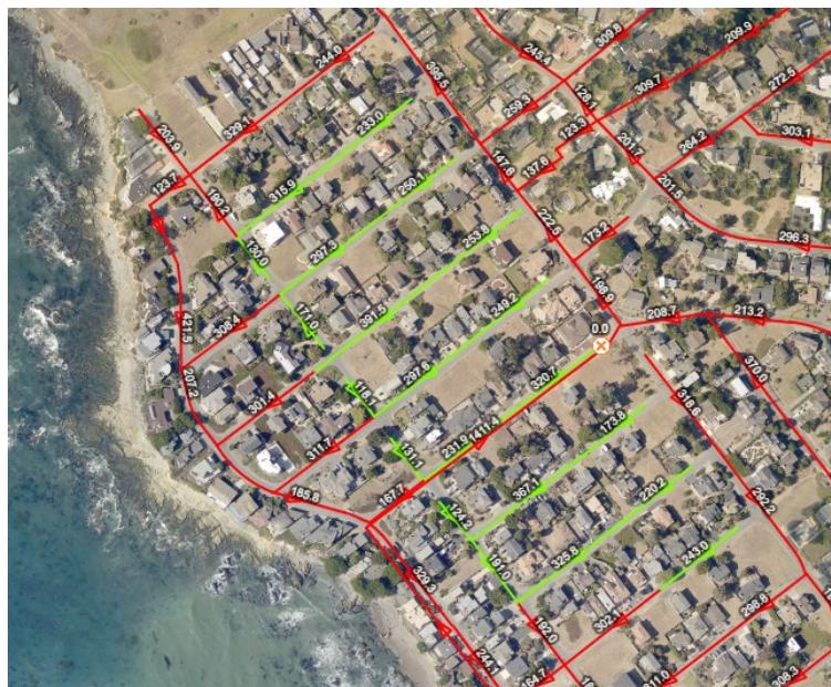
Figure A - Screenshot of sewer line preventative maintenance layer in GIS
