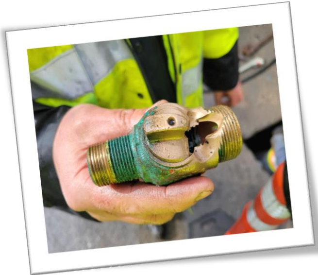
Pictured Left: ¾" Service line 3' below the surface leaking at 3 GPM
