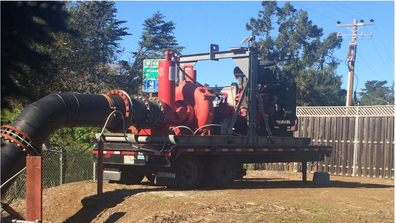
Flood Pump on Main Street - West Village
