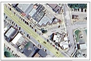
The current parking pattern in West village is 60 deg. angle, about 9 ft wide and about 20 ft. from curb to end is about 20 ft. This would be used where possible.
