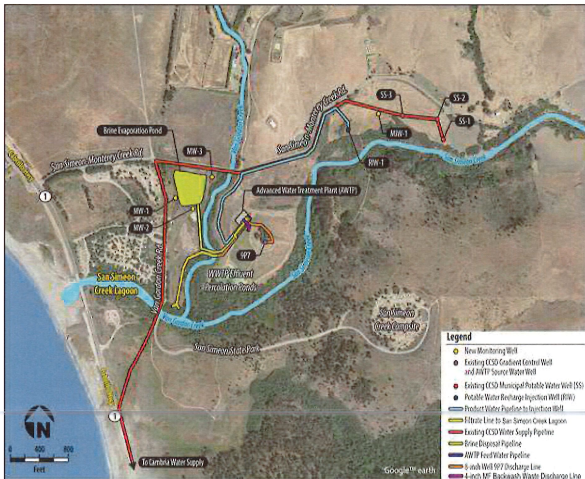
Figure 3 - Emergency Water Supply Project (Extraction Well, Treatment Plant, Percolation Ponds, Title 27 Impoundment, Groundwater Injection Site, Water Supply Wells)
